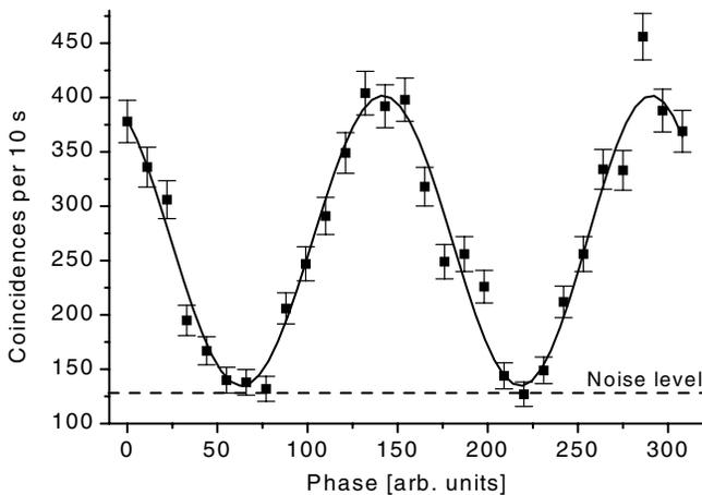
FIG. 2. Two-photons interference fringes. According to a sinusoidal fit, the visibility is  $97\% \pm 5\%$  after subtraction of the accidental coincidences.
