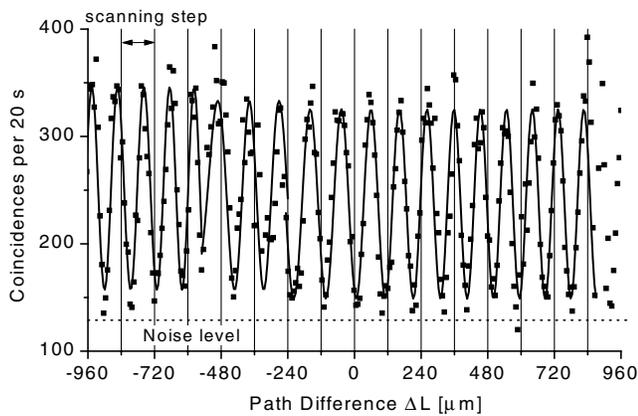
FIG. 3. Two-photon interference fringes. The total scan was done on a range of  $\pm 3$  mm, but for more clarity the figure shows only a range of  $\pm 1$  mm around the estimated equilibrium point. Each vertical line grid corresponds to a step of the scan. No disappearance of the correlation is observed.
